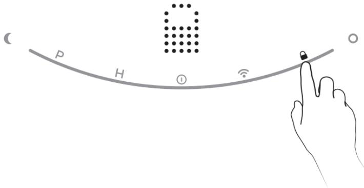
Long press the “lock” button to enable child lock.
