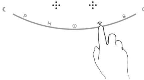
Long press (3 seconds) below Wi-Fi icon to activate "I'm listening" mode on aair lite and connect device to Wi-Fi.
