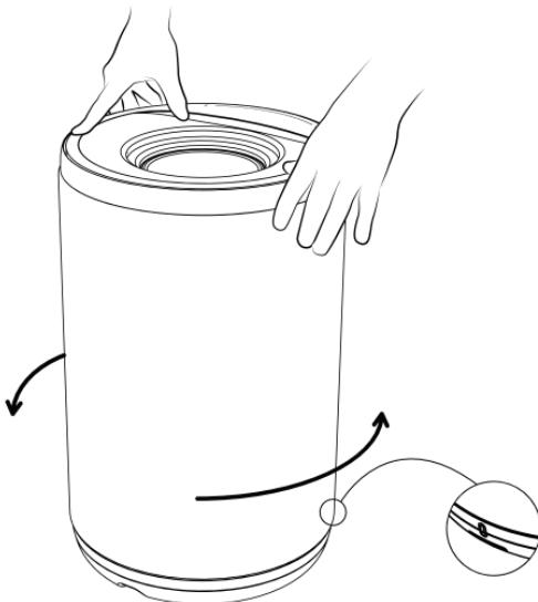
Lift off the upper cover from the device and pull out the main filter by pressing the clips on each side. Slide in a new filter until you hear a click. Close the device with the cover.
